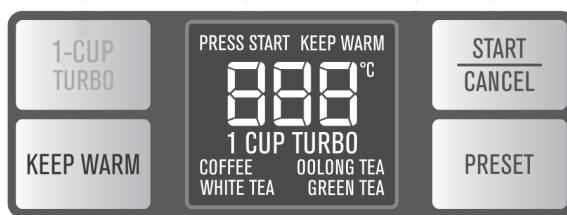
**1-CUP TURBO button:** Boils quickly 200ml of water in less than one minute\*.
