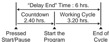
After selecting Delay End time, press Start/Pause touchpad to start the program. Machine will then countdown and update time on the display every hours until it reaches the starting point of the wash cycle.
