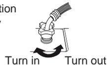
The inlet hose must not be lengthened. If it is too short and you do not wish to move the tap, you will have to purchase a new, longer hose specially designed for this type of use.
