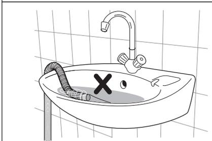
In this case, make sure the end cannot come unhooked when the machine will be emptied. This could be done by tying it to the tap with a piece of string or attaching it to the wall.
