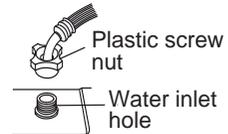
6. Turn in the plastic screw nut to tighten the connection of the water supply hose with the water inlet hole.
