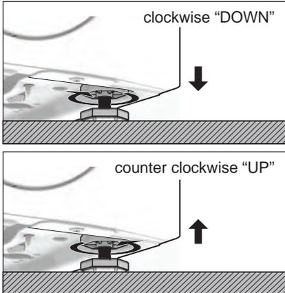
When the machine is levelled, try to rock it from corner to corner. If it does rock, adjust the legs again until it is levelled and does not rock.
