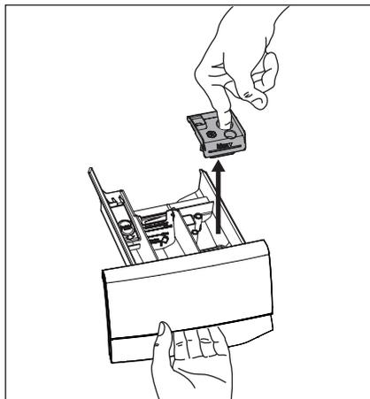
Flush it out under a tap to remove any traces of accumulated powder.
